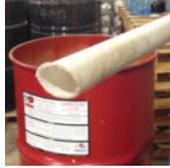
1. CUT PICKUP TUBE AT AN ANGLE
