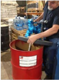
3. AFTER SECURING PICKUP TUBE, SET THE PUMP ASSEMBLY LID ON TOP OF DRUM
